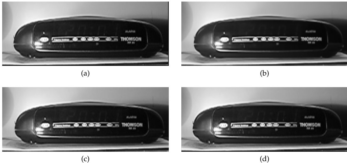
Figure 5.4: Images produced by robust methods for clock sequence. (a) Our original projective method, (b) l_1 norm method with bilateral TV regularization, (c) the median gradient method of Zomet with bilateral TV regularization, and (d) the projective method with a previous median filter applied.
