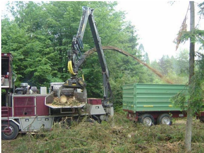
**Figura 4.8:** Astilladora transportable.
