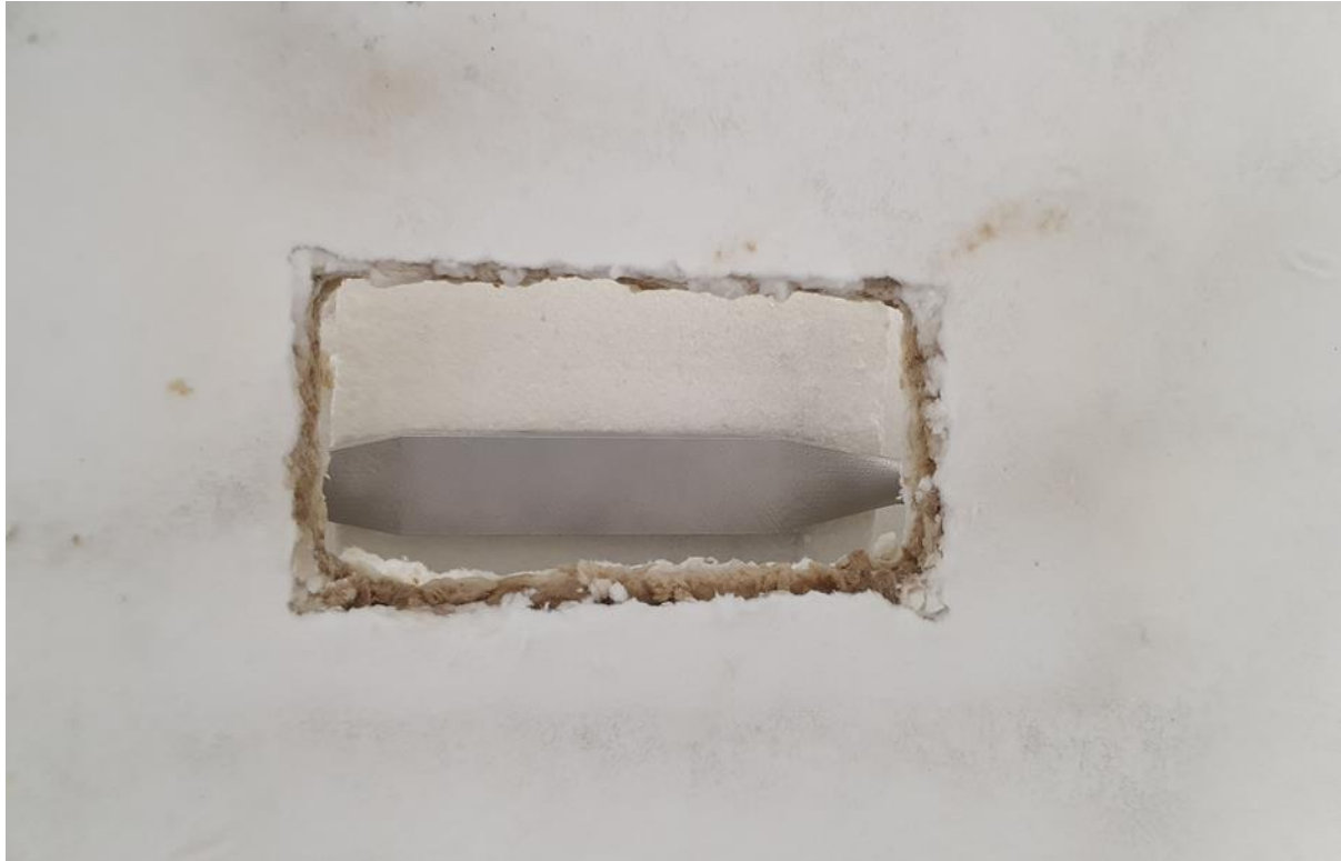
Figure 68. Alumina radiation shield around receiver as on 11/08/2022 (before experiment)
