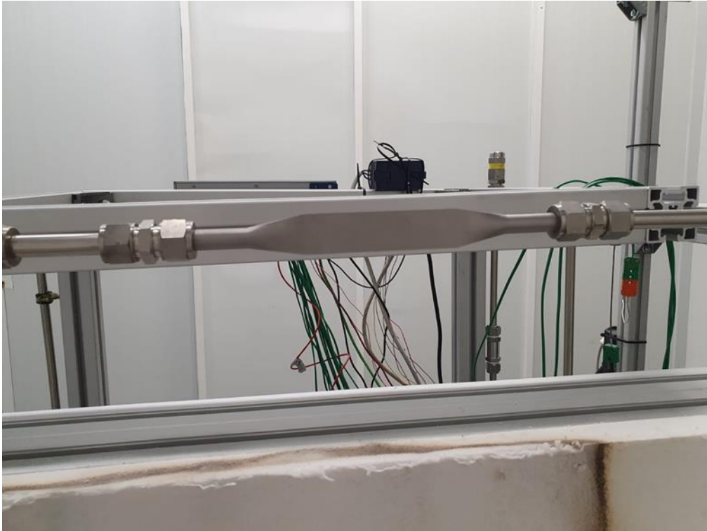
Figure 65. PR1 geometry receiver installed in testbed as on 03/08/2022.
