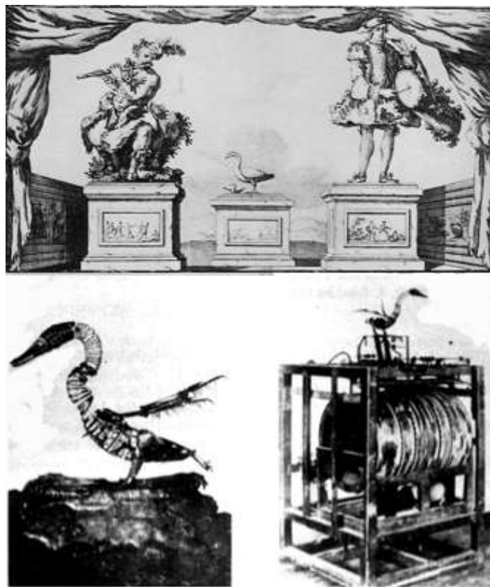
Fig. 1.2 – Above: drawing from a leaflet of Vaucanson's time of three of his most famous automata: the flute player, the mechanical duck and the tambourine player. Below: two XIX century pictures of the now lost mechanical duck, supposed to replicate all the living animal functions, including digestion (from Chapuis & Droz 1949).
