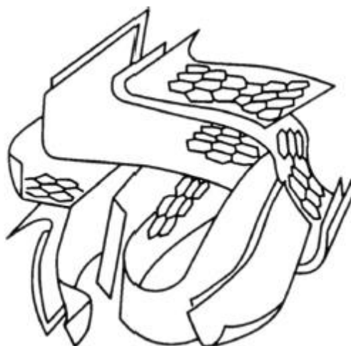
Figure 1.17 Schematic representation of activated carbon turbostratic microstructure. 113
