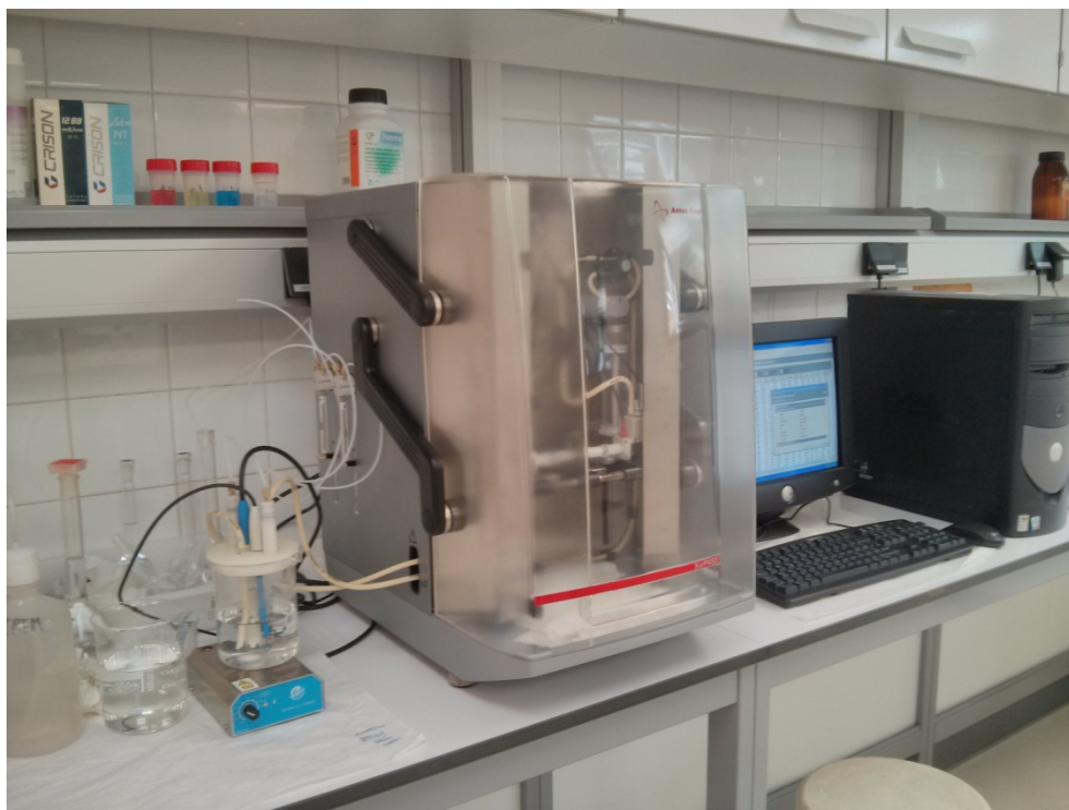
Fig.8.7. Medidor potencial Z SurPASS electrokinetic analyzer (Anton Paar GmbH).
