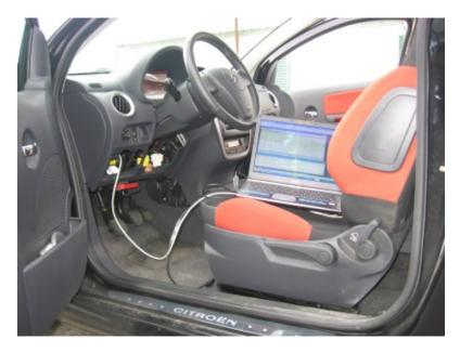
Figure 7. Analyzer software tool connected to the OBD connector in a Citroen C2
