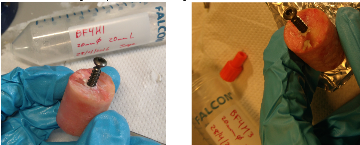
Figure 24. Example of screw insertion in bovine bone cylindrical samples.
