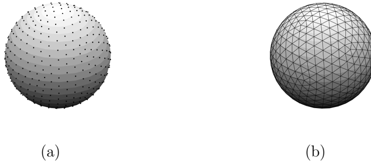
Figure 2.3 Spherical sampling. Spherical deconvolution methods use a sampling strategy that relies on probing the signal at evenly distributed points over a unit sphere: (a) sampled points; (b) faces defined by the edges linking the sampled points. There are many solutions to the issue of packing points on a sphere. In this case, the number of points (vertices) is V = 492 and the number of faces F = 480 .
