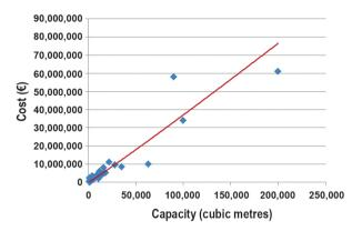
Figure 5. Ratio between storm water tanks capacity and cost.
