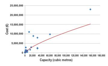
Figure 4. Ratio between storage facility capacity and cost.
