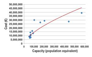
Figure 6. Ratio between large WWTPs capacity and cost.
