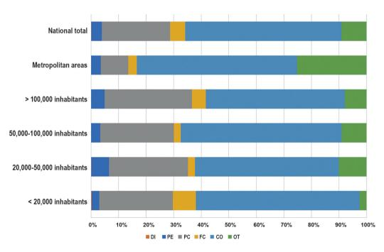
Figure 2. Sanitation network distribution, broken down by material and stratum.
