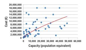
Figure 7. Ratio between smaller WWTPs capacity and cost.
