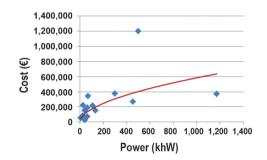
Figure 8. Ratio between pumping stations installed power and cost.
