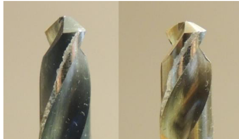
Fig. 8. Adhesions in drills number 16 (on the left) and 8 (on the right)
