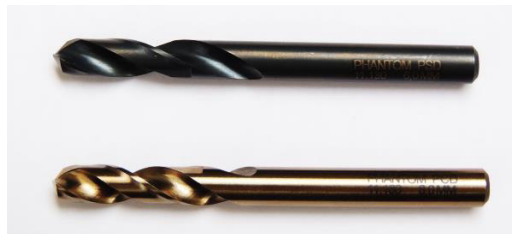
Fig. 1. Drills with point angles of 118^\circ (on the top) and 135^\circ (on the bottom).
