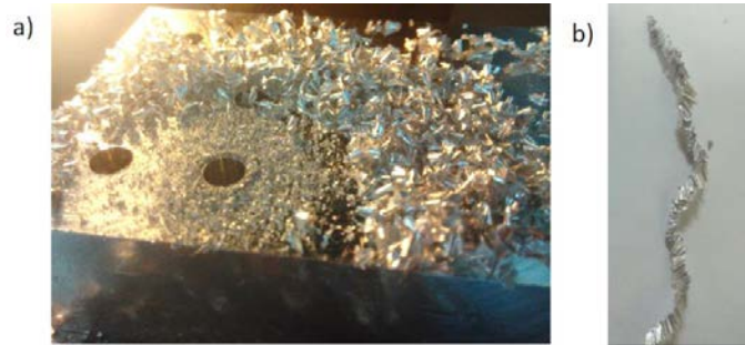
Fig. 7. Chips obtained in drills number a) 5, b) 32.
