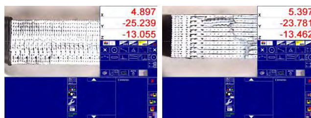
FIGURE 7. View of the cross section of two test specimen for tensile testing with horizontal position (left) and edgewise position (right). Images obtained by TESA-VISIO Digital Profile Projector.
