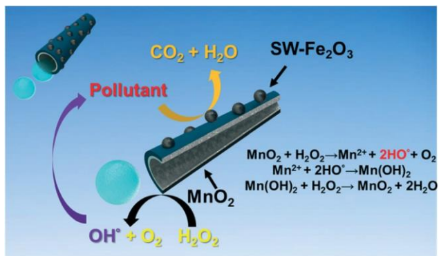
Fig. 1 Schematic representation of the micromotors based advanced oxidation of anthraquinone dyes and chlorophenols into environmentally friendly products and related radical's generation mechanism. Please note that \text{Mn}^{2+} represent an intermediate of the reaction that occurs in the surface of the catalyst. As such, \text{Mn}^{2+} is not released in solution.
