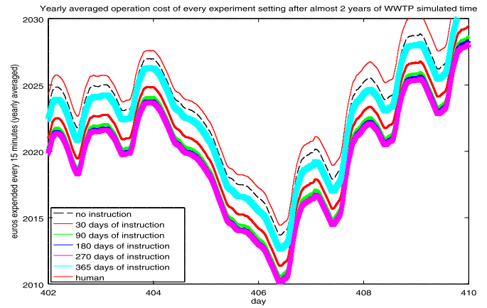
Fig. 7. Yearly averaged operation cost of each of the 7 settings; around a year of simulated time.
