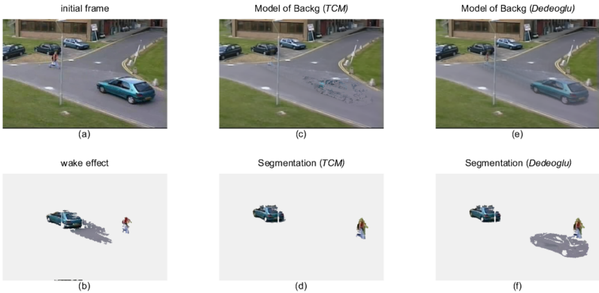
Figure 13. Qualitative comparison of the capacity to react to eliminate ghosts using the truncated cone method (TCM) and the strategy proposed by (Dedeoglu, 2004). (a) Frame no. 608, initial frame, (b) example of increased reactivity, which can be achieved with both methods, at the expense of bad segmentation, (c) frame no. 634, elimination of the ghost from the background model and (d) from the segmentation output using the TCM, (e) frame n° 634, ghost remains in the background model and, therefore, (f) it is still present in the segmentation output according to the strategy proposed by Dedeoglu.
