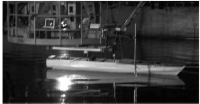
Figure 10. Scaled down replica 1/25 the size of a high-speed ferry in El Pardo Model Basin (Spain).
