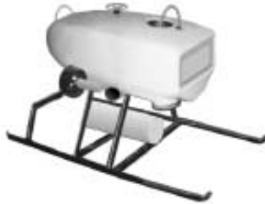
Fig. 13 The simplified CAD model of the Garbí, used for matching with the real image
